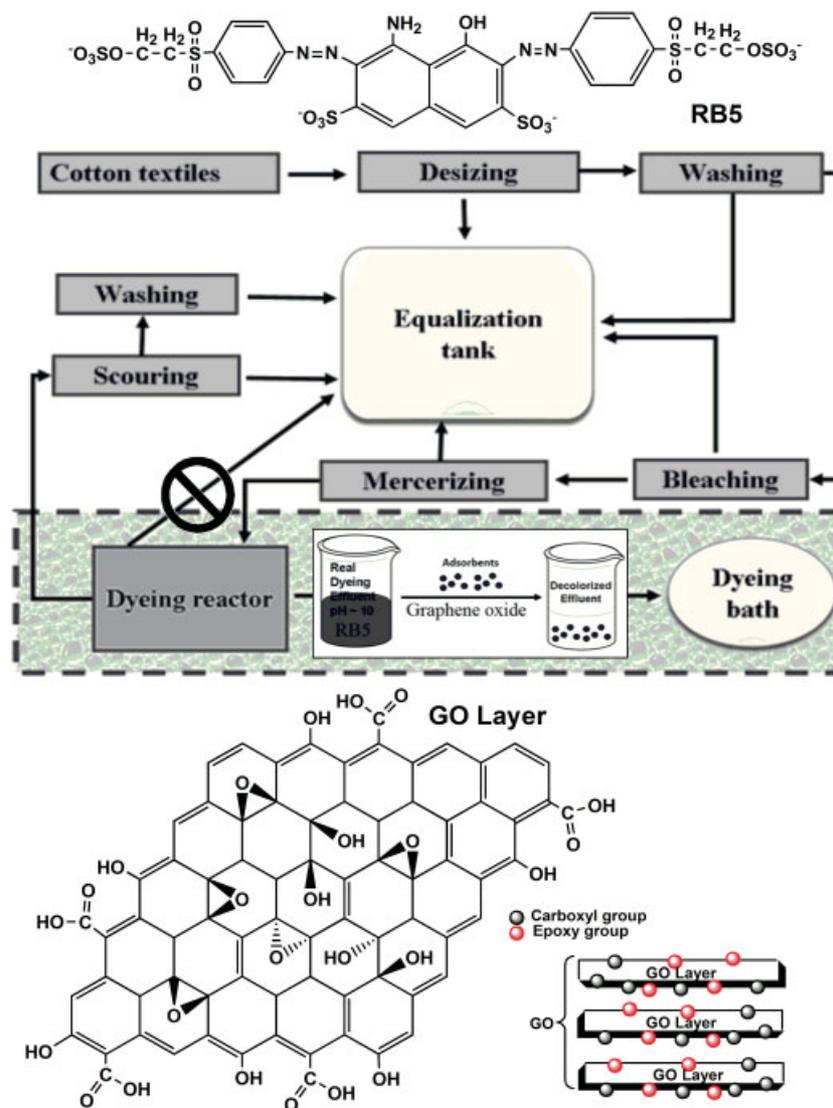
**Figure 1.** Illustrative scheme of the dyeing process and the proposed treatment of its effluents; RB5 dye (top) and functionalized GO adsorbent (bottom).
