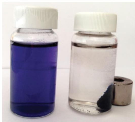
**Figure 2.** Image of the magnetic graphene oxide nanoparticles (synthesized by co-precipitation) adsorbing RB5 dye; on the right, following magnetic separation. Reprinted with permission; copyright MDPI AG (2012).<sup>16</sup>
